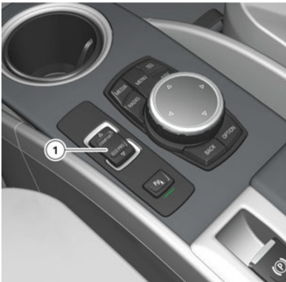
Switch block with driving experience switch
